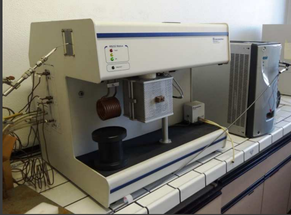
Micromeritics Autochem II 2920 BET, TPR, TPD, O 2 -TPD, Outlet connected with a Quadrupole Mass Spectrometer ESS- Genesis
